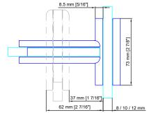
Glass Thickness = 8-12mm [5/16" to 1/2"] Max. Door Leaf Weight = 75kg [165 lbs] Max. Door Leaf Width = 1000mm [39 3/8"]
