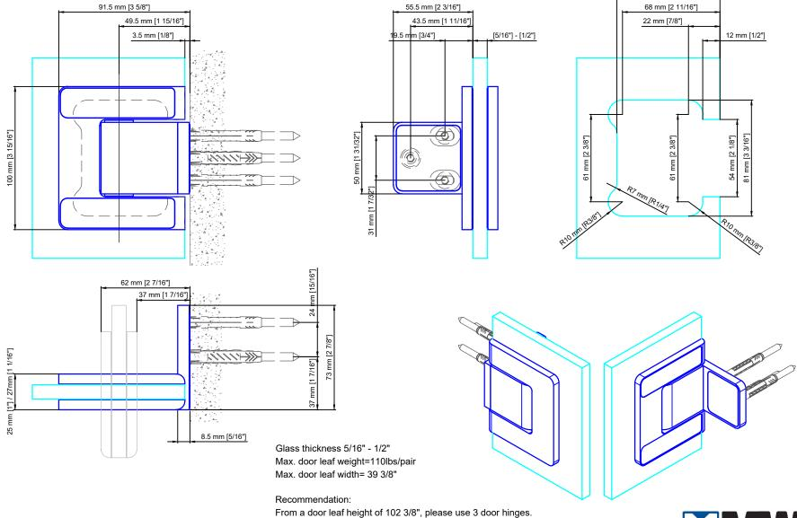
Installation of the additional door hinge in the upper third of the door.
