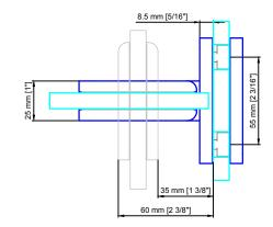
Glass thickness = (8 / 10mm) ([5/16"] / [3/8"]) Max. Door Leaf weight =50kg [110lbs] / pair Max. Door Leaf width = 1000mm [39 3/8"]
