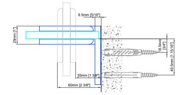
Glass Thickness: 8-10mm [5/16"]-[3/8"] Max. Door Leaf Weight= 50kg [110lbs] per pair Max. Door Leaf Width= 1000mm [39 3/8"]
