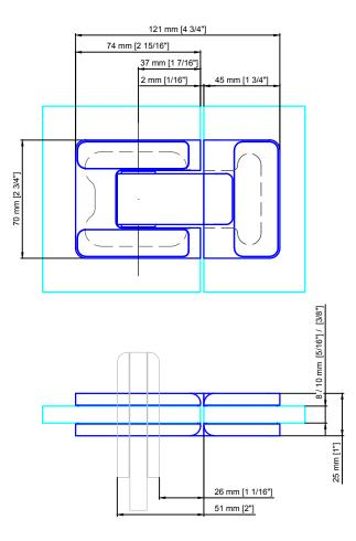
Glass thickness 8-10mm / [5/16"] [3/8"] Max. door leaf weight=50kg [110lbs"]/pair Max. door leaf width= 1000mm [39 3/8"]
