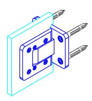
Glass thickness: 8 - 10mm / [5/16"] - [3/8"] Max. door leaf weight= 110lbs/pair Max. door leaf width= 1000mm [39 3/8"]
