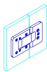
Glass thickness: 8 - 10mm / [5/16"] - [3/8"] Max. door leaf weight= 110lbs/pair Max. door leaf width= 1000mm [39 3/8"]
