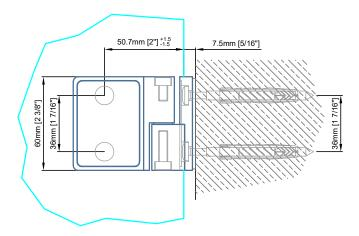
Shown in the open position. Door lifted max. 4mm [3/16"]
