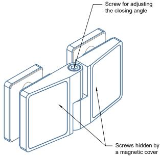
\*See specification Lifting Hinge [DD.0100 L/R] Glass to Glass -180° for dimensions without seal
