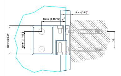
Shown in the open position. Door lifted max. 4mm [3/16"]
