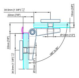
Shown in the open position. Door lifted max. 4mm [3/16"]
