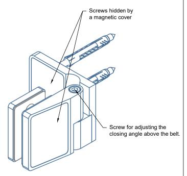
\*See specification Lifting Hinge [DD.0110 L/R] Glass to Wall - 90° with seal
