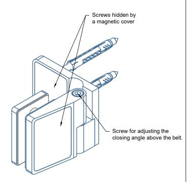
\*See specification Lifting Hinge [DD.0110 L/R] Glass to Wall - 90° for dimension without seal
