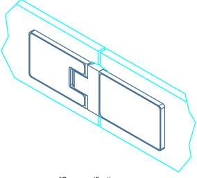
\*See specification Pivot Hinge [DD.3392 L/R] Glass to Glass - 180° for dimension without seal
