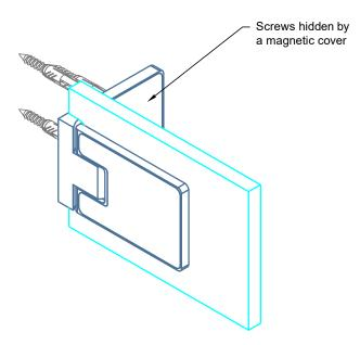
\*See specification Pivot Hinge [DD.3390 L/R] Glass to Wall - 90° with seal
