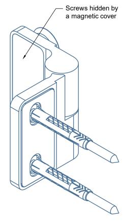
\*See specification Pivot Hinge [DU.3342] Glass to Wall] - 90° with seal
