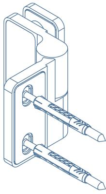
\*See specification Pivot Hinge [DU.3343] Glass to Wall] - 90° with seal
