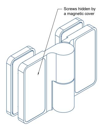
\*See specification Pivot Hinge [DU.3341] Glass to Glass] - 180° with seal
