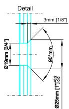
Shown in the open position. Door lifted max. 6mm [1/4"]
